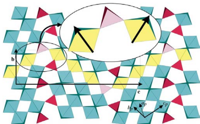
Figure 18 Type of tilting observed in \text{P}_4\text{W}_{12}\text{O}_{44} ( P2_12_12_1 ). In a chain of polyhedra (represented in yellow), the tilting (symbolized by arrows) always takes place in the same direction.
